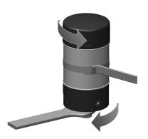
Examine bottom section, especially sealing surfaces, for mechanical damage.
